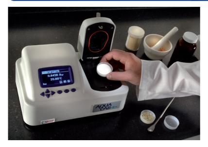
Water Activity (or ERH) is a measure of the free water available for mould growth and bacteria. It influences a product's shelf life, odour, colour, flavour and texture. The AquaLab is used to determine and control the optimum water activity to produce the highest quality product with the least amount of preservative.
